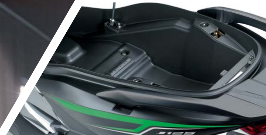
UNDERSEAT STORAGE WITH HYDRAULIC OPENING STRUT AND LED COURTESY LIGHT
